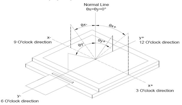
Note (2) Definition of Contrast Ratio(CR): measured at the center point of panel
